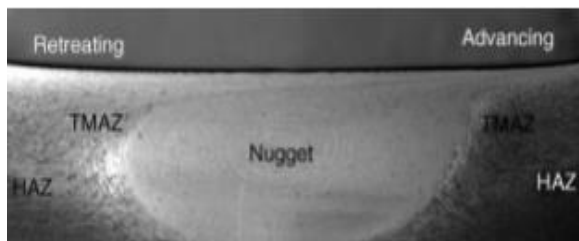
Fig 4: A Macrograph Showing Various Microstructural Zones in FSP 7075Al-T651 (Standard Threaded Pin, 400 rpm and 51 mm/min). [1]
